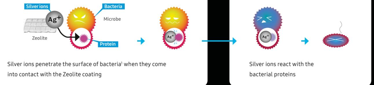
Silver ions penetrate the surface of bacteria<sup>1</sup> when they come into contact with the Zeolite coating
